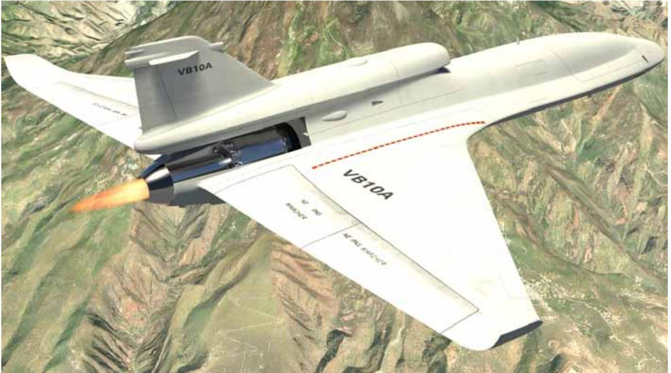
An excellent power-to-weight ratio, compact design, reliable operation, low fuel and oil consumption together with starting at high altitudes and at high speeds make PBS jet engines stand out among competing engines.
