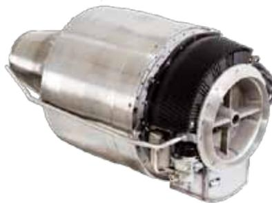
(1,250 N thrust). It is a single-shaft engine composed by a starter generator integrated in the radial compressor impeller, one axial turbine, autonomous oil system and digital control system. To this day almost 1,000 units have
